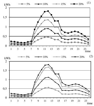
Figure 14. Standard deviation of hourly energy losses for the scheme with renewable generation and with reconfiguration (1), and without renewable generation and with reconfiguration (2).
