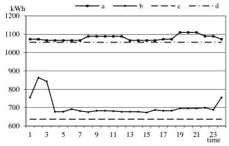
Figure 7. Comparison of daily power losses at constant configuration of distribution network without renewable generation - a, and with renewable generation - b, with daily losses obtained for optimal reconfiguration without renewable generation - c and with renewable generation - d.
