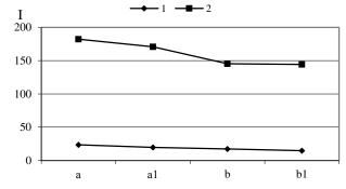
Figure 10. Minimum 1 and average 2 voltage (U), average 1 and maximum 2 currents (I) in tie lines, a — without renewable generation and without reconfiguration, b - without renewable generation and with reconfiguration, a1— with renewable generation and without reconfiguration, b1- with renewable generation and with reconfiguration.
