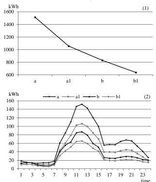
Figure 6. A change in the daily (1) and hourly (2) power losses in distribution network with and without reconfiguration and presence of renewable energy sources, a – without renewable generation and without reconfiguration, a1 – without renewable generation and with reconfiguration, b –with renewable generation and without reconfiguration, b1 – with renewable generation and with reconfiguration.
