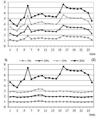
Figure 15. Errors in the determination of hourly energy losses for the scheme with renewable generation and with reconfiguration (1), and without renewable generation and with reconfiguration (2).
