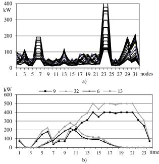
Figure 4. Variation in active power of loads at the nodes of distribution network, Fig.1 (a) and active power of renewable energy sources (b) during a day.
