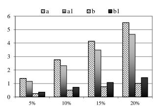
Figure 16. Standard deviations (a, a1) (kWh) and errors (b, b1) (%) of daily energy losses for the network with renewable generation and with reconfiguration (a, b), without renewable generation and with reconfiguration (a1, b1).
