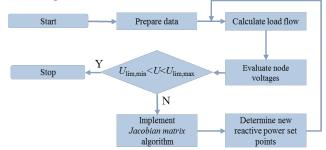
Fig. 2. Iterative optimization method for grid support
