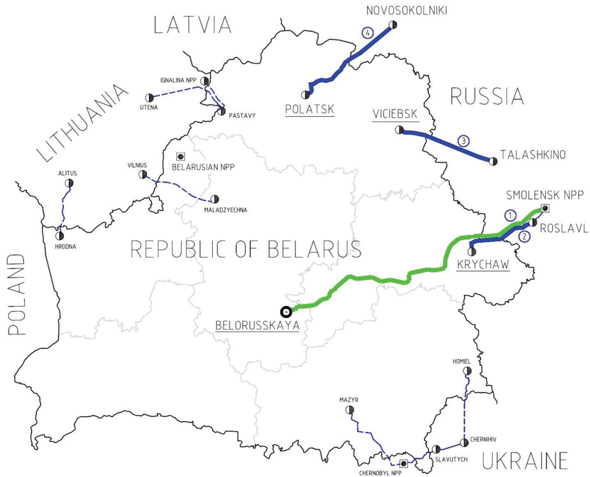
Fig. 1. 330 kV and 750 kV transmission lines connecting the Belarusian power system with the UES of Russia.
