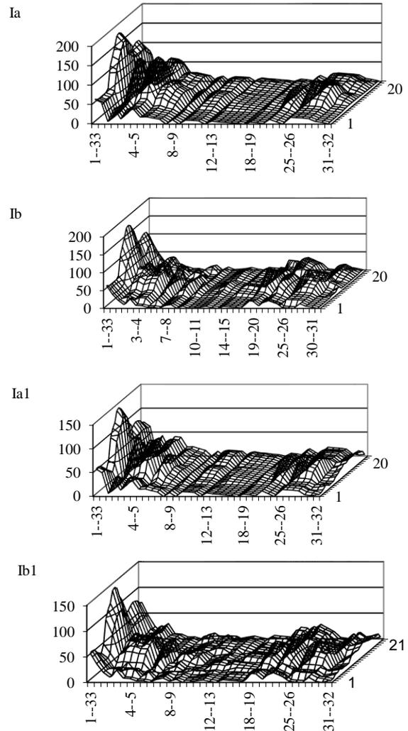
Figure 9. Hourly variations in voltage at nodes and current in branches of the test network with and without reconfiguration and renewable generation, Ua, Ia – (voltage and current) without renewable generation and reconfiguration, Ub, Ib – without renewable generation and with reconfiguration, Ua1, Ia1 – with renewable generation and without reconfiguration, Ub1, Ib1 – with renewable generation and with reconfiguration.
