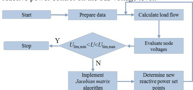
Fig. 2. Iterative optimization method for grid support
