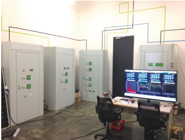
Fig. 4. A smart grid test bench at the laboratory of energy systems at Skoltech. Every rack contains a load (either linear or nonlinear) or generator (of different types).
