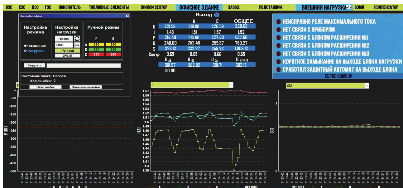
Fig. 5. A screen capture from the SCADA system of the test bench. It is clear that only the RMS values of voltages and currents can be seen.
