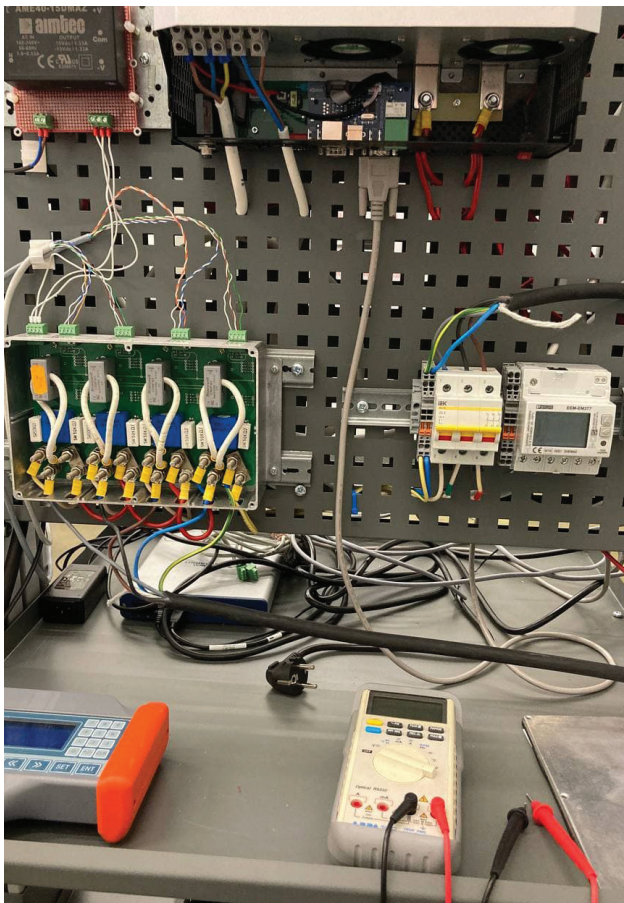
Fig. 7. High resolution sensors mounted on a rack and plugged-in to the smart grid test bench.
