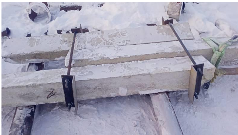
Fig. 5. The way of fastening the ballast to transfer the test load to the footings.
