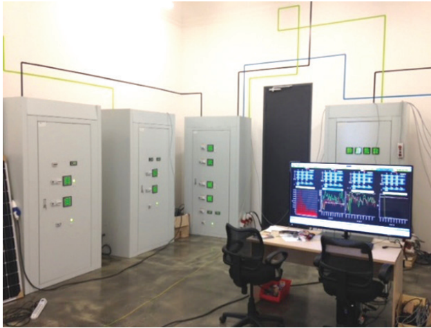
Fig. 4. A smart grid test bench at the laboratory of energy systems at Skoltech. Every rack contains a load (either linear or nonlinear) or generator (of different types).
